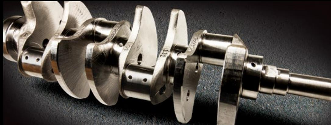
“This is essentially an all-new powertrain that’s unique to GT350, and it takes full advantage of the new Mustang platform’s outstanding chassis dynamics. Make no mistake, the engine is an American interpretation of a V8 with flat-plane crankshaft, and it produces a distinctive, throaty howl from its four exhaust tips.”
